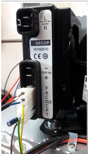
On ACC02 there is a cable marked with «A». This has to be connected to the «A» and the other one to «C»
