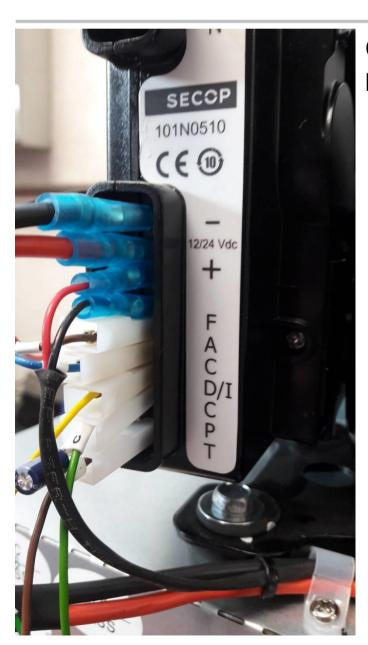
Connect the red cable of the fan on «+» of the power supply
