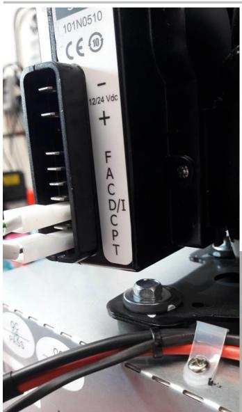
Connect the green cable of ACC01 on «C» and the brown cable on «T»
