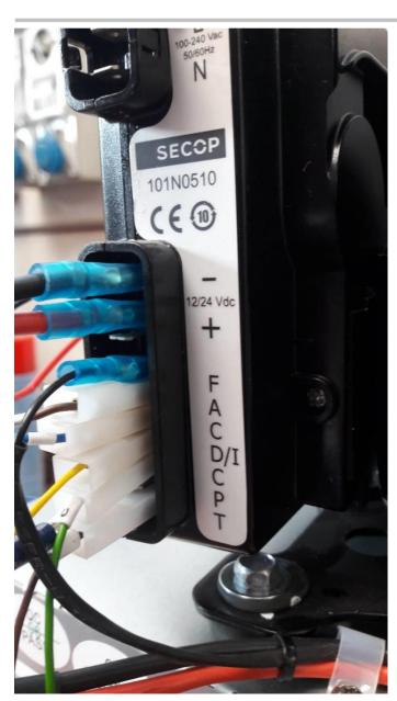
Connect power supply to the ECU, red cable on «+» and black cable on «-»
