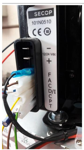
Connect the black cable of the fan to «F» on the ECU
